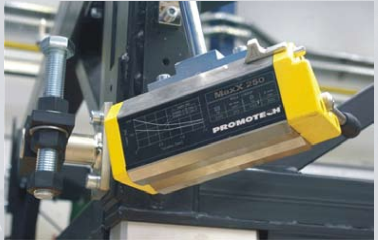
6 top quality permanent magnets provide workholding system 6x 250kg which ensures firm, fast & easy machine job to job re-positioning.
