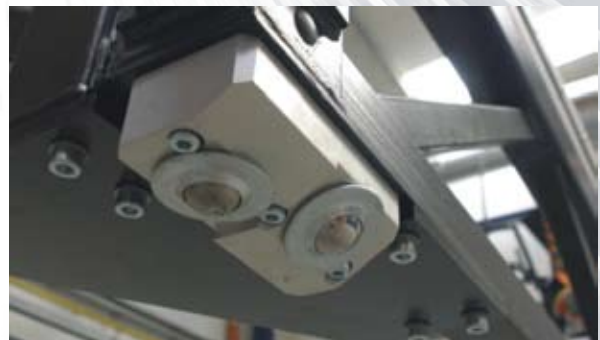
Roller balls make sliding inside can section much easier.
