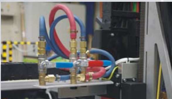
Quick action valve within hand's reach enables fast on/off switch of fuel gas supply to the torch
