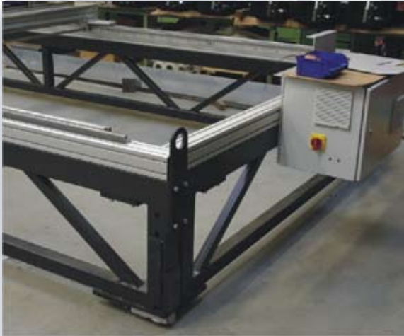
Heavy duty steel & aluminum frame with increased rigidity
